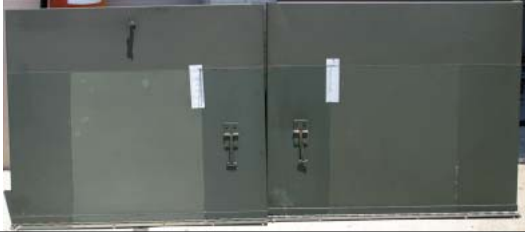
Figure 1 – Side by side comparison of panel with chalked coating removed and not removed
