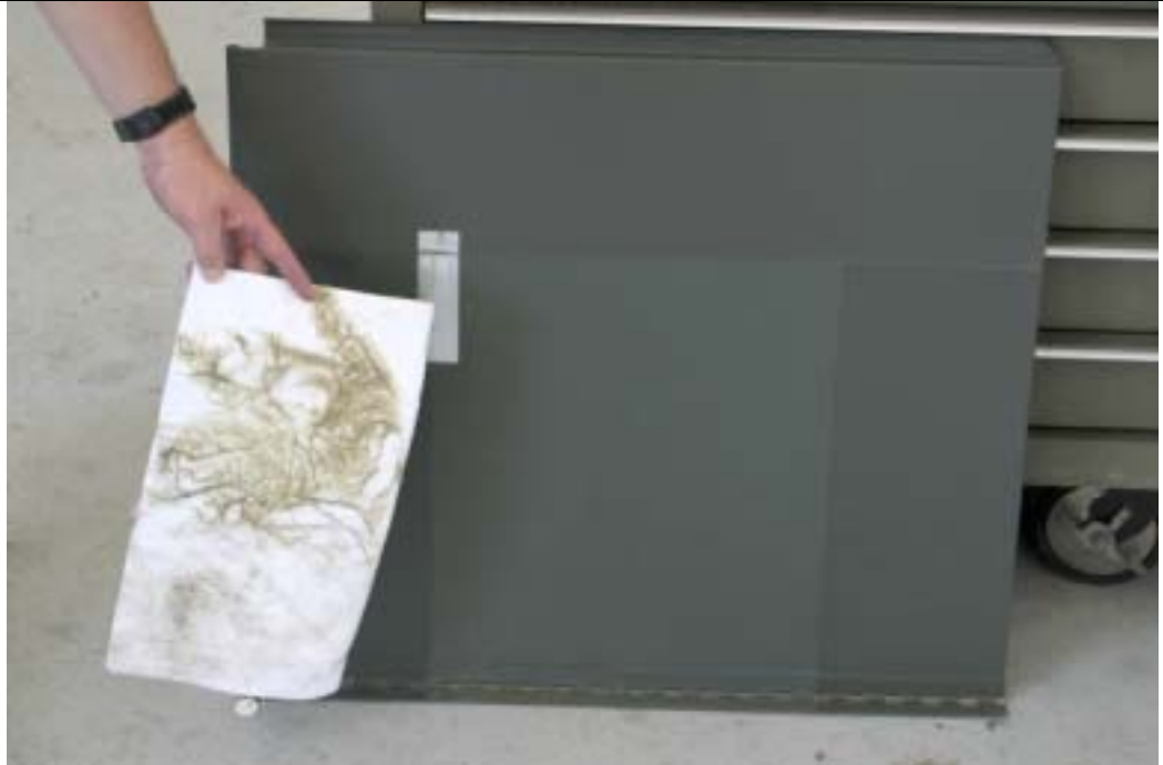
Figure 2 – Chalked 0-VOC coating removed
