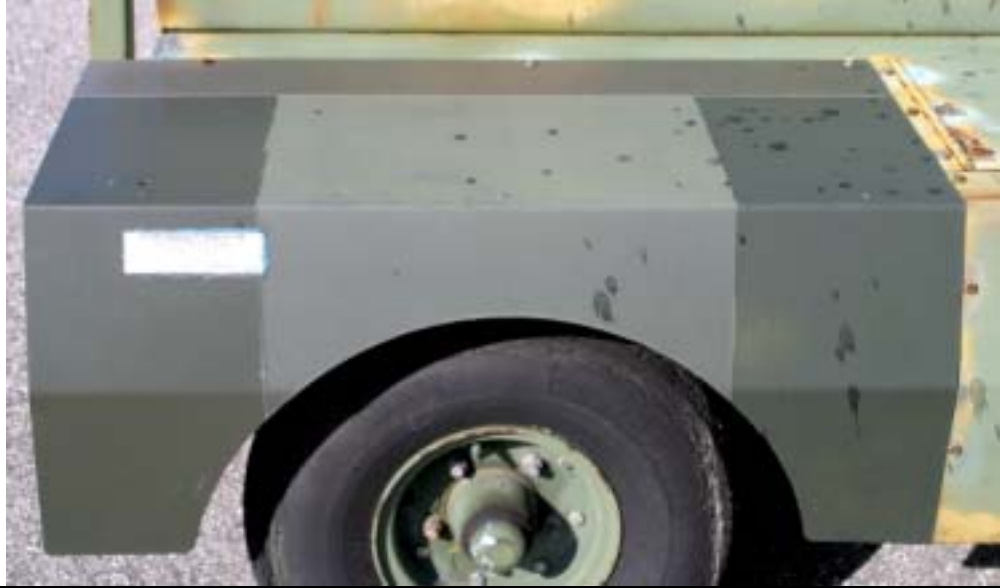
Panel 3 – Typical color/shade variation noted on all of the 0-VOC coating, semi-gloss green test panels
